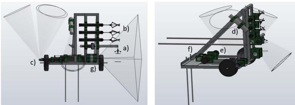
Figure 1. Drawing of the WEST platform (©DynamOcean). Instruments placed on the platform (with letters referenced in the text). Insonified areas are represented with circles.
