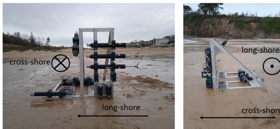
Figure 2. Deployment of the WEST mooring at Porsmilin, on February 28<sup>th</sup> 2022 (©France Floc'h). Cross-shore and long-shore directions are indicated for clarity.
