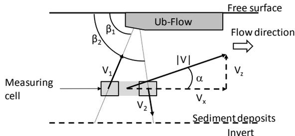
Figure 3: Schema of measurement cell and Ub-flow position at free surface
