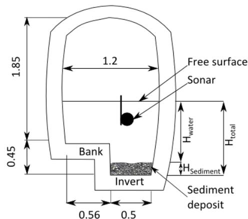
Figure 1: Collector geometry
