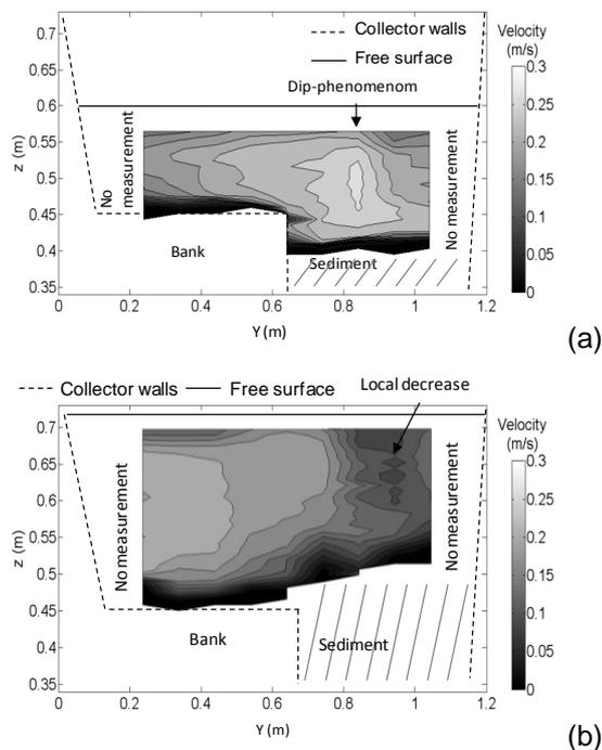
Figure 7: Transversal variation of longitudinal velocity, (a) 10/10/2013 measurements and (b) 11/20/2013 measurements
